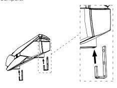
Slide Bracket Tabs into Slots in Rubber Bumpers
