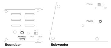
NOTE: The maximum wireless operating distance between the soundbar and subwoofer is approximately 50 feet (15.3m).
