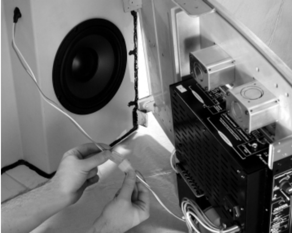
Figure 8: Connecting the Subwoofer Driver
