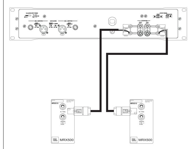
\*MRX512M: Input panel has the same number of connectors, but are located at either end of the enclosure.
