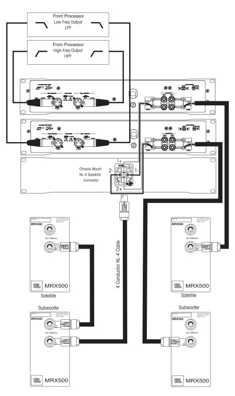
Using 4-Conductor Cable, Subwoofer configured for Pins 2±. (See Block Diagram)
