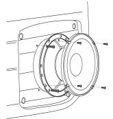
**NOTE:** The CS2106 uses an adaptor to fit a variety of different 6" openings. Select an appropriate adaptor ring and secure it to the vehicle using the sheet-metal screws provided, then attach the speaker to the ring with the machine screws.
