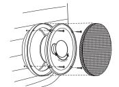
**Figure 4.** Mounting the CS2106 in a 165mm speaker location.
