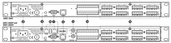
SDEC-3000 has no CobraNet or Word Clock connections, but is otherwise identical to the SDEC-4000P and SDEC-4000X.
