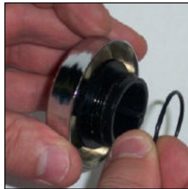
Replacing the O-ring
