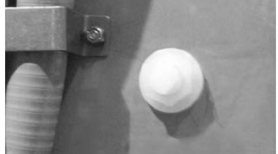
Detergent Connection Point (Machine rear view)
