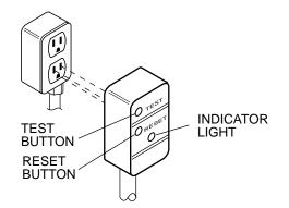
1. The spa is supplied with a 15 foot line cord which terminates with an integral GFCI plug. Locate the spa near enough to a weather protected outlet, but no closer than 10 feet. DO NOT USE AN EXTENSION CORD! Using an extension cord is hazardous and will decrease the amount of power to the unit, causing slow heating, poor whirlpool performance, or system malfunction.
