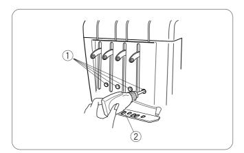
Apply a few drops of oil to the needle bar throgh the holes in the front cover.
