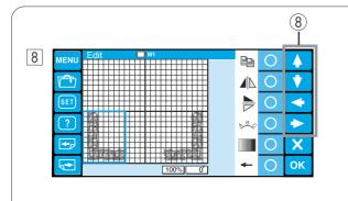
8 Move the flipped pattern to the left bottom corner of the editing screen by using the arrow keys or by dragging it with your fingertip.
