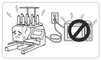
Do not use the machine near appliances that radiate electromagnetic noise such as a microwave oven, or do not plug in the machine to the same branch circuit where such appliances are connected.
