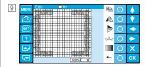
Make a duplicate of the pattern and flip it vertically. Move the flipped pattern to the top left corner of the editing screen.
