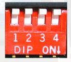
**Non-Navigation Radios:** Dipswitch 2 MUST be set in the **ON** (down) position for proper operation.
