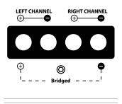
J2-360.2 is designed to deliver power into speaker loads equal to or greater than 2 ohms per channel when using a "stereo" configuration and speaker loads equal to or greater than 4 ohms when using a "bridged" configuration.
