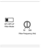
1) "Filter Mode" Control: The J2-360.2 employs a 12dB per octave filter. This filter can be configured into one of two filter types or defeated completely by way of the threeposition "Filter Mode" switch:
