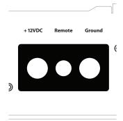
The amplifier will turn on when +12V is present at its "Remote" input and turn off when +12V is switched off. If a source unit does not have a dedicated remote turn-on output, the amplifier's turn-on lead can be connected to +12V via a switch that derives power from an ignition-switched circuit.
