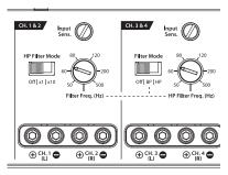
1) "Filter Mode" Controls: The XD700/5 employs 12dB per octave filters for each pair of main channels (one high-pass filter for channels 1&2 and another high-pass / bandpass filter for channels 3&4. The Subwoofer Channel provides a low-pass filter with the option of 12dB or 24dB / octave slopes. Each of these filters can be controlled or defeated completely by way of the three-position "Filter Mode" switches in each Channel Section:
