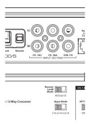
If you wish to send six discrete channels into the XD700/5, simply use all six inputs and set the "Input Mode" switch in the "6 Ch." position. The amplifier will automatically combine the Sub Ch. input signals to mono.
