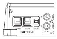
The XD700/5's "+12 VDC" and "Ground" connections are designed to accept 4 AWG power wire. 4 AWG is the required wire size for this amplifier.
