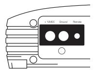
The e1200's "+12 VDC" and "Ground" connections are designed to accept 8 AWG - 4 AWG power wire. 8 AWG is a minimum power wire size for this amplifier.
