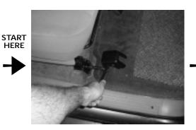
**STEP 1:** Using a 14mm socket, remove the four bolts that secure the passenger side front seat.
