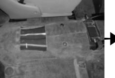
\*Tundra Access Cab Only\* STEP 12: Cut 1-1/2" off of each carpet flap, that is located in front of the mounting holes, from STEP10.
