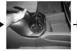
**STEP 4:** With the main storage door open, grab ahold of the black cup holder section and pull up.
