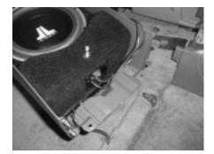
**STEP 21:** Place the Stealthbox/center console into vehicle. Attach the speaker wire to terminal. Back out the three socket cup screws to 1-1/4:".
