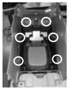
**STEP 9:** Remove the 8 screws that is securing the black plastic support to the outer console. Not all circles represent all 8 screws.
