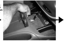
**STEP 7:** Slide the center console to the rear of truck. This will allow exposer of the 12v plug wires. Unplug and then remove the center console from truck.
