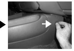
**STEP 6:** Remove the plastic buttons that are located on each side of the center console.
