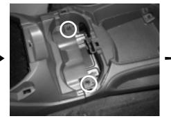
**STEP 5:** Using a 10mm socket, remove the exposed bolts. Also remove the bolts that are located at the bottom of the main storage bucket.
