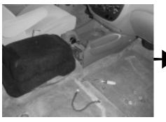
**STEP 19:** With the Stealthbox and the modified A/C ducts in position. Place the front section of the center console back into the proper location. Do not secure at this time.
