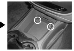
**STEP 3:** Remove the front storage access door. Using a 10mm socket, remove the exposed bolts.
