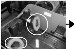
**STEP 8: \*Tundra Access Cab Only\*** With the center console out of the truck, flip up side down. Remove the two air duct ears that are located to the rear of the center console.
