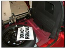
**STEP 3** Remove foam filler panel from passenger side of spare tire.
