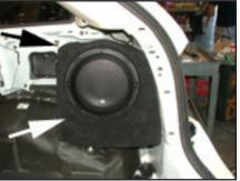
**STEP 13** Place Stealthbox® into location as shown, push stud against wax square to make an impression in the wax square.
