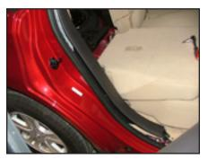
STEP 6 Pull passenger side cargo panel away from the door jamb.
