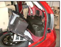
STEP 7 Remove passenger side cargo panel by prying away from side of vehicle and floor.
