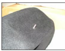
**STEP 15** Extend mounting stud 1 1/2 inch from enclosure.
