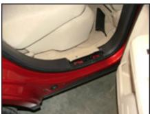
STEP 5 Remove passenger side threshold plate.
