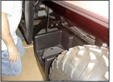
STEP 4 Set the enclosure on the ground in front of the drivers side rear wheel oriented as shown.
