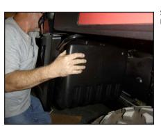
STEP 5 Lift the enclosure up onto the previously installed bracket.
