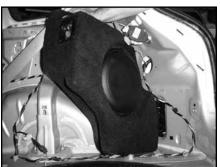
**STEP 7**Position the Stealthbox® into place.
