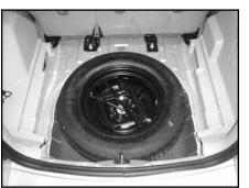
**STEP 3**Pull the plastic flooring and rear sill plate out.
