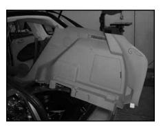
**STEP 4**Remove the right side rear cargo panel out of the car.
