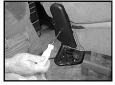
**STEP 2:** Remove the black plastic covers from each side of the armrest, of the center seat.
