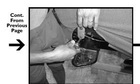
**STEP 13:** Attach the plastic clips on the Stealthbox upholstery to the bars under the seat structure.
