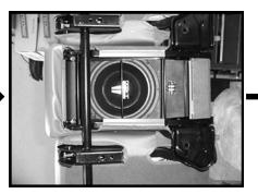
**STEP 14:** Run speaker wire from the amplifier to the Stealthbox mounting location. Be sure the wires are routed in such a way that they will not be pinched when the seat is reinstalled.
