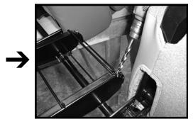
**STEP 9:** Bolt the supplied brackets to the the Stealthbox using two of the bolts removed from the armrest in Step 3. Do not tighten these bolts yet.
