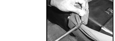
**STEP 10:** Place the Stealthbox on the seat frame where seat cushion was removed from. Be sure the two studs in the front edge of the Stealthbox fit into the two holes drilled in Step 8.
