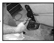
**STEP 3:** Remove the four Torx bolts that attaches the armrest to the center seat.
