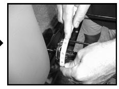
STEP 7: Measure 2 1/4" from the front lip of the center seat structure side bars. Make a mark at the 2 1/4" measurement.
