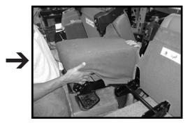
**STEP II:** Thread the supplied nuts on the two studs and tighten securely.
