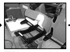
**STEP 5:** Remove the upholstery from the lower center seat by releasing the four plastic clips holding it in place.
