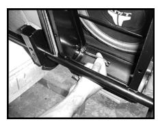
**STEP 12:** Using the two remaining factory bolts from the armrest bolt the brackets on the Stealthbox to the seat structure. Tighten all bolts securely, including those installed in Step 9.
