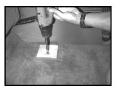
STEP 8: \*Double check under the truck for brake lines, fuel lines or any other wiring.
