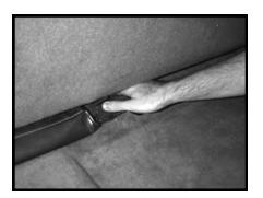
**STEP 2:** Under the rear bench seat, there are a pair of metal brackets which hold the tire changing tools. Bend these up and back so they are out of the way of then enclosure.
