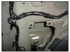
**STEP 9**This shows the holes where the bracket mounts.
