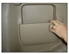
**STEP 1**Remove the cover in front of the pocket as shown.
