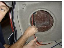
Remove the woofer from the Stealthbox®. Hold the enclosure in place and use a marker to mark the interior panel through the hole in the back of the Stealthbox®
