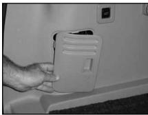
**S T E P 3 4** Reattach the wire harness to the power lift gate switch and access door from **STEP 6**.
