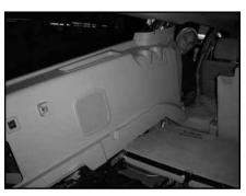
**STEP 19** Remove the side panel from the SUV.
