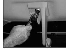
STEP 6 Remove the access door from the driver's side rear cargo panel.
