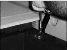
STEP 5 With an 8mm socket, remove the pair of bolts that secure the lift tray to the floor.
