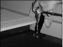
**STEP 37** Secure the lift tray to the floor, from **STEP 5**.
