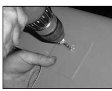
**STEP 31** With a drill and a 1/8-inch drill bit, drill through the impression made in each wax square and into the vehicle's side panel.
