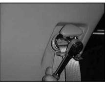
STEP 11 With a T-50 torx socket, remove the bolt that secures the driver's side second row seat belt to the c-pillar.
