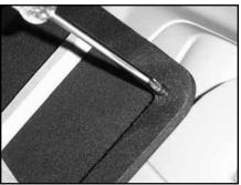
**STEP 29** Mount each supplied Phillips head screw into each corner of the backside of the supplied grille, as pictured.
