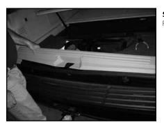
**S T E P 3** Remove the tailgate's lower sill plate.
