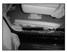
**STEP 14** Remove the driver's rear door sill plate.
