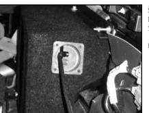
**STEP 27** Run speaker wire from the amplifier location to the Stealthbox<sup>®</sup> location.
