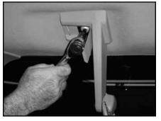
**S T E P 3 6** Secure the third row seat belt to the ceiling and floor, from **STEPS 8 & 9**.
