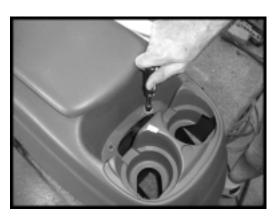
**STEP 7:** Run speaker wire to the mounting location of the Stealthbox. Trim to length and attach to the Stealthbox.
