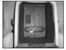
**STEP 2:** Remove tray and liner to reveal two 18mm bolts. Remove these bolts. Remove console from truck.
