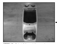
**STEP 13:** Reinstall the outside console over the inner console and the Stealthbox with eight 7mm bolts which were removed in steps 6,7 and 8. Place the conlose/Stealthbox back into the truck.
