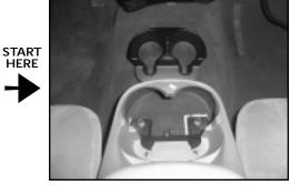
**STEP 1:** Remove the front cup holder to reveal two 18mm bolts. Remove these bolts.
