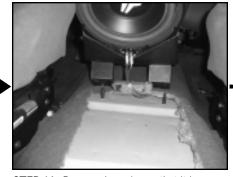
**STEP 14:** Run speaker wire so that it is accessible at the front of the enclosure, connect it to the enclosure and test for proper operation.
