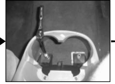
**STEP 15:** Using an an 18mm socket wrench, secure the front of the console to the vehicle with the 18mm bolts removed in Step 1.
