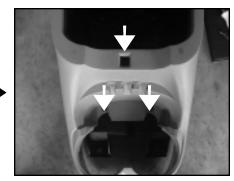
**STEP 7:** Remove three 7mm bolts denoted by the arrows in the picture.
