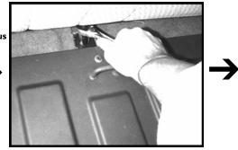
**STEP 5:** Place the rear seat back into the truck. Start securing the plate by bolting in the two bolts that were removed in **STEP 2**.
