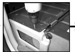
**STEP 6:** Replace and secure all eight T-30 bolts, that were removed in **STEP I**.
