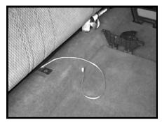
**STEP 4:** Run speaker wire to the enclosure location. At this time, check the woofers for proper operation.
