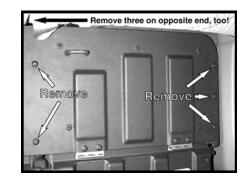
**STEP I:** Flip the rear seat up, this will expose the metal plate that needs to be removed. With a T-30 socket, remove the 8 factory bolts.
