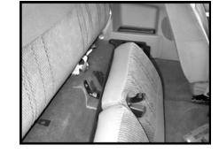
**STEP 3:** With all the mounting bolts removed, remove the rear seat.
