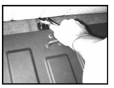
**STEP 2:** Remove the two bolts that secure the panel to the rear of the cab, with a 18mm socket.
