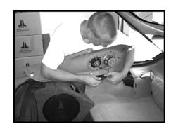
**STEP 8:** Reconnect the factory speaker wires and replace the driver's side trim panel over the enclosure.
