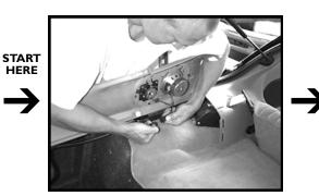
**STEP I:** Remove the driver's side trim panel, disconnect the speaker wires, if applicable.
