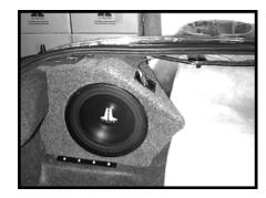
**STEP 5:** Run speaker wires to the enclosure. At this time, check the woofer for proper operation.
