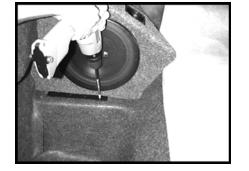
**STEP 4:** Using the supplied four self-tapping screws. Seucre the enclosure's moutning bracket to the flooring of the vehcile.
