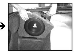
**STEP 3:** Insert the enclosure into the cubbyhole, taking care to loft and tuck the wiring harness above the enclosure as you slide as you slide it in. Push the enclosure firmly into place
