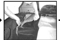
**STEP 2:** Remove the driver's side carpet from the cubby-hole in the corner of the hatch. this piece of carpet will not be used in the installation. Vehicle owner should keep this carpet for possible future use, when removing the Stealthbox.
