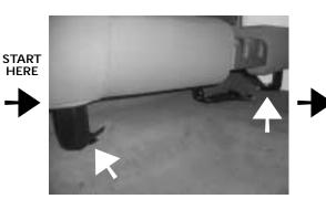
**STEP 1:** With an 18mm deep socket, remove the two front mounting nuts. Also remove the jack out of the metal holder.
