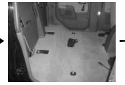
**STEP 5:** Remove the rear seat out of the vehicle. You should use a second person to help out.
