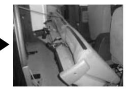
**STEP 3:** With the rear mounting nuts removed, tilt the rear seat forward, off the mounting studs.
