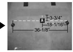
**STEP 6:** Place the middle of the supplied wax square, in the middle of the mounting studs and 3-3/4" from the point of the floor as it starts to elevate up. Remember to remove the paper backing.
