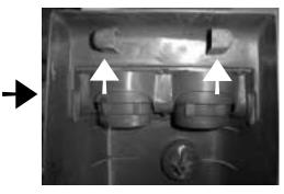
**STEP 12:** On the back side of the plastic jack cover, there are two plastic guides.
