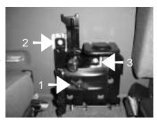
**STEP 3:** Remove the (1) tire stops and with a 10mm socket, (2&3)unbolt the jack bracket.
