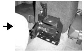
**STEP 8:** With the supplied hardware, attach the jack bracket to the front of the Stealthbox.
