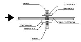
**STEP 11:** Attache the jack bracket to the floor, using the supplied hardware.
