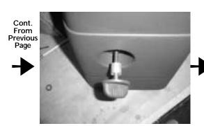
**STEP 13:** Place a supplied 3/4"Lx3/4"ODx3/8"ID spacer onto the thumb screw.
