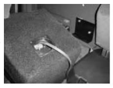
**STEP 6:** Attach speaker wire to the Stealthbox terminal and check the woofer for proper operation.
