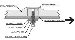
**STEP 16: (Outside the vehicle)** Place the supplied hardware in order onto the exposed socket cup screw. If more exposed threads are needed, back out the socket cup set screws.
