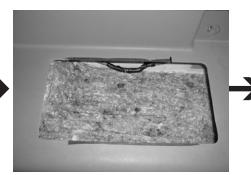
**STEP 9:** (Inside the vehicle) Cut and remove the factory jute(sound deadening), from the removed storage area, from **STEP 5**.
