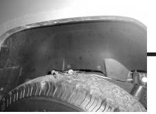
**STEP 7:** With the plastic trim out of the way, remove the plastic inner wheel well.
