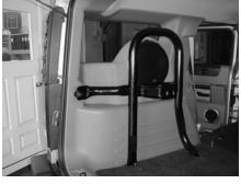
**STEP 22:** With the spare tire rack properly positioned, it should not interfere with the enclosure.
