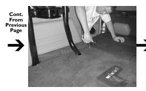
**STEP 23:** Replace the jack and the jack tools, that were removed in **STEP 3**.
