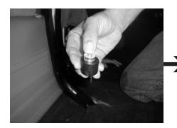
**STEP 19:** With the spare tire rack placed into position. Loosely tighten the lower factory bolts to the lower mounting feet.
