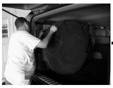
**STEP 24:** Secure the spare tire onto the rack and replace the tire cover.
