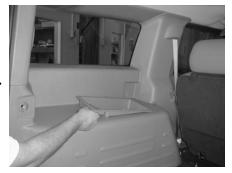
**STEP 5:** By pulling up, remove the driver's side rear storage bucket.
