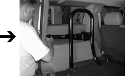
**STEP 4:** With an 8mm socket, remove the four bolts that secure the spare tire rack.
