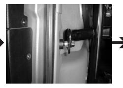
**STEP 20:** Placed A supplied spacer, between each upper mounting foot of the spare tire rack and the side panel.
