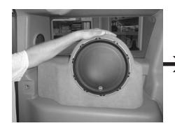
**STEP I1:** Thread the supplied pair of socket ca set screws into the enclosure, leaving 1/2" exposed. Place the enclosure into place and firmly press
