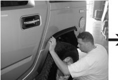
**STEP 17:** Mount the plastic inner wheel well and plastic trim from **STEPS 6 & 7**.
