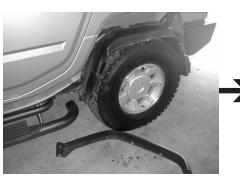
**STEP 8:** Rest the plastic inner wheel well on the rear tire. Keep the trim and all the mounting hardware together.
