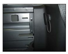
**S T E P 4**With a Phillips screw driver, remove the two screws that secure the driver's side c-pillar to the rear wall.
