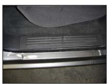
**STEP 5**Pull off the driver's side rear door sill plate.
