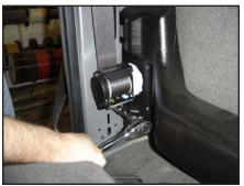
With a T-45 socket and ratchet, remove both the passenger's side and the driver's side seat belt retracting units.
