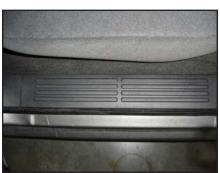
**STEP 3**Pull off the passenger's side rear door sill plate.
