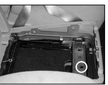
STEP 7 Remove the plastic tray from vehicle.
