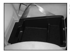
STEP 6 Grab a hold of the bottom cushion and pull forward. Remove the bottom cushion from the vehicle.
