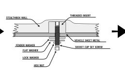
STEP 7: Back out the/each socket cup set screw to expose about 1-1/2".
