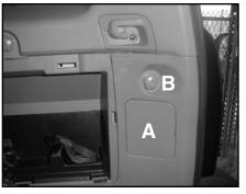
**STEP 8:** Remove the access door(**A**) and cargo net cleat(**B**).
