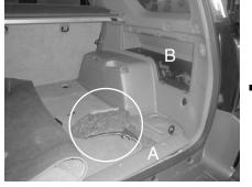
**STEP 2:** Remove the rear sill plate(A) and side storage door(B).
