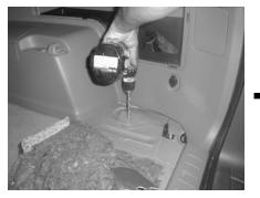
**STEP 5:** With the Stealthbox removed and wax square still in position, use a 1/2" drill bit to drill out the marked location.
