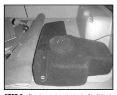
**STEP 9:** Run the speaker wire to the Stealthbox's location.
