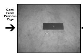
**STEP I1:** Take the other supplied black metal plate, lock washer, flat washer and nut to the under side of vehicle.
