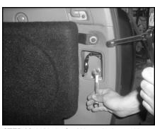
**STEP 10:** With the Stealthbox wired up and in location(with socket cup set screw placed through the carpet, metal plate and floor).
