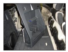
**STEP 12**Secure the driver's side plastic panel back onto the rear wall.
