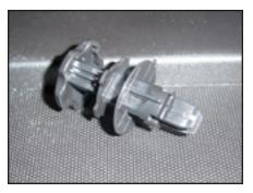
**S T E P 6** There are two anchors for cargo in the upper corners of the rear plastic trim panel. These two anchors need to be removed in order to remove the trim panel. To remove these, pull on the outside of the anchor top section it will pull out, allowing the anchor itself to collapse and be pulled out.
