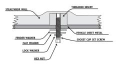
**STEP 8:** With the socket cup set screws protruding through the floor of the vehicle. Place the supplied fender washer, flat washer, lock washer and hex nut in this order.
