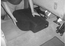
**STEP 4:** Place the enclosure into position and press down firmly.
