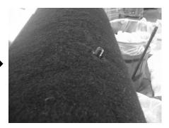
**STEP 3:** Place the supplied socket cup set screw into the enclosure, leaving 1/4" exposed.
