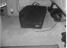
**STEP 7:** Run and attach speaker wire from the amplifier location to the enclosure.
