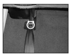
**STEP 4**Remove the bolt that secures the seat belts to the floor.
