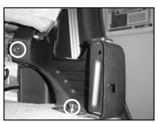
Remove the two bolts that secure the mounting foot to the rear bulkhead and floor.
