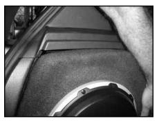
**STEP 4.A**The Stealthbox® needs to fit all the way to top plastic panel.
