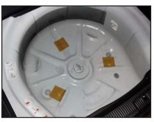
STEP 7 The three 3/8-16 x 2-1/4" Set Screws should have made a mark in the wax squares as shown.
