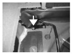
**STEP 6:** Look to the front left of the cargo area for the two factory bolts that are securing a black plate to the floor.
