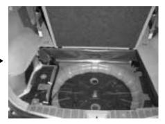
STEP 3: a) With a Phillips® screw driver, remove the driver's side cargo pocket. **b)**Unsnap the wiring harness that is running
