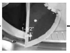
**STEP 16: a)** Flip over the side floor panel. Measure 1-1/2" from the outside left edge to the right. This measurement needs to line up with the round dual lock fastener position markings made in **STEP 15**. Mark the final location.
