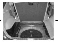
STEP 2: Open the cargo flooring and hook it to the upper lip of the tailgate opening. Remove the organizer tray, wooden board, factory woofer enclosure, spare tire and the driver's side cargo pocket cover.
