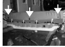
STEP 4: This picture is looking from the backseats to the tailgate opening, showing the tailgate sill plate.
