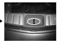
STEP 5: With a small flat blade; pop out the oval plastic cover of the tailgate sill plate, that is located under the tailgate hook latch.
