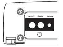
The A1800's "+12VDC" and "Ground" connections are designed to accept 4 AWG power wire. 4 AWG is a minimum power wire size for this amplifier.
