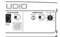
1) "Filter Mode" Control: The A2150 employs a 12dB per octave filter which can be configured into one of two filter types or defeated completely by way of the three-position "Filter Mode" switch:
