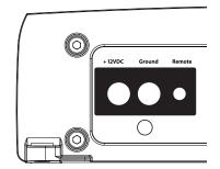
The A4300's "+12VDC" and "Ground" connections are designed to accept 8 AWG - 4 AWG power wire. 8 AWG is a minimum power wire size for this amplifier.
