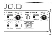
1) "Filter Mode" Control: The A4300 employs a 12dB per octave filter for each pair of channels (one filter for channels 1&2 and another filter for channels 3&4). Each of these filters can be configured independently into one of two filter types or defeated completely by way of the three-position "Filter Mode" switches:
