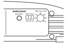
The el 400D employs a sophisticated, variable, low-pass active filter for its internal channel. This feature is designed to attenuate frequencies above its filter frequency, so that the system's subwoofers do not reproduce any audible midrange content.
