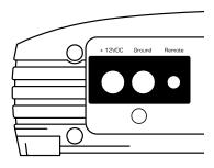
The e1400D's "+12 VDC" and "Ground" connections are designed to accept 8 AWG - 4 AWG power wire. 8 AWG is a minimum power wire size for this amplifier.
