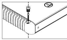
The standard method of mounting requires removal of the four corner caps with the 3/16-inch hex wrench included with your amplifier. Using appropriate mounting screws (not included), secure the amplifier in all four corners and replace the corner caps.
