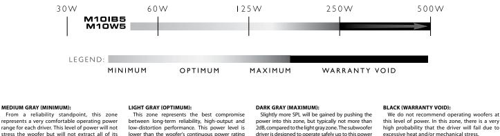
excessive heat and/or mechanical stress. Subwoofer drivers operated at these levels of power are NOT covered under warranty.
