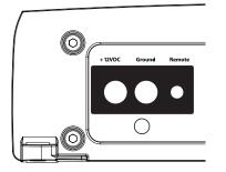
The A1400's "+12VDC" and "Ground" connections are designed to accept 4 AWG power wire. 4 AWG is a minimum power wire size for this amplifier.
