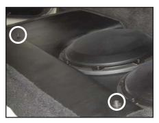
**STEP 1**Thread the supplied socket cup screws into the bottom of the Stealthbox®, leaving 1/2-inch of the threads exposed.
