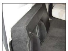
**STEP 2** Place the Stealthbox® into the truck, like in the picture.
