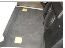
Remove the paper backing from the supplied wax squares. Eye ball the placement of the wax squares onto the floor with the Stealthbox® placed into the truck.
