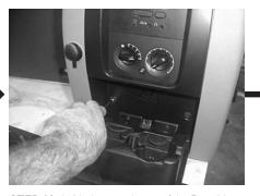
**STEP 12:** With the console out of the Expedition, pull down the rear cup holders. Us e a 7mm bolts that have been exposed.
