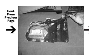
**STEP 23:** Use a OEM bolt that was just removed to plug the driver's side bolt hole.
