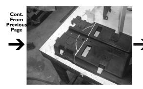
**STEP 15:** Cut out the template that is found on **Page 6**. Place this template across the rear portion of the black inner console. Mark the correct scribe lines.
