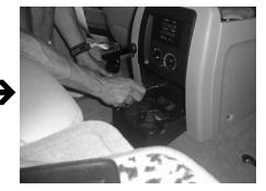
**STEP 30:** Secure the rear outer console, from **STEP 12**.
