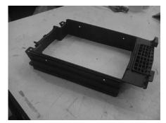
**STEP 31:** Taking the factory storage bucket, Cut to allow for a new depth of only 3-1/8", from the top edge.
