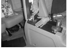
**STEP 32:** Secure the storage lid from **STEP 6** and front passenger seat if you did remove.
