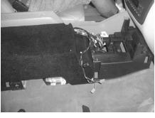
**STEP 26:** Place the front portion of the modified black inner console, in front of the enclosure.
