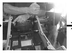
**STEP 13:** Using a 17mm socket, remove the bolts that secure the outside walls to the inner black console.
