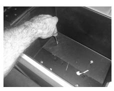
**STEP 3:** In the center console, remove the rubber liner. Using a 7mm socket, remove these four bolts.
