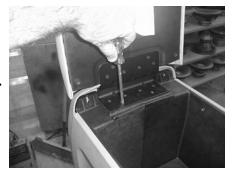
STEP 6: With a screwdriver remove the six screws that secure the console lid.
