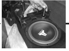
**STEP 20:** Using the supplied hardware of (2) 3/8"-16 x 1" hex bolts, (2) 3/8" flat washers and (2) lock washers. Attach this drilled out position of the black console, to the rear of the enclosure.
