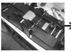
**STEP 16:** Scribe cut lines on the front portion of the black inner console. Using the picture as a guide. Same side as the scribe lines from **STEP 15.**
