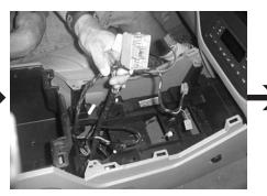
**STEP 9:** Once the wire harness is unsecured, disconnect the white plug.
