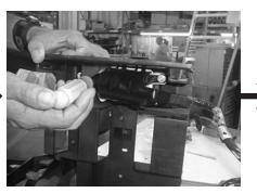
**STEP 25:** Using a 7mm socket, secure the wire harness that was removed in **STEP14**.
