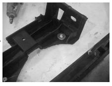
**STEP 18:** With the rear portion of the black console, now modified. Place the supplied pair of washers, tucked in the corners. Mark washer's inner holes and then remove the washers
