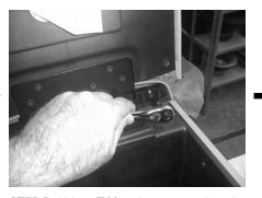
**STEP 5:** Using a T-20 socket, remove the pair of bolts at the top corners of the storage bucket.
