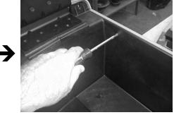
STEP 4: With a screwdriver remove the four screws that are found around the top edge of the storage bucket.
