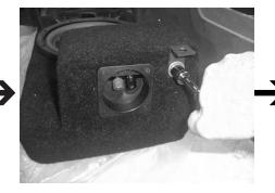
**STEP 21:** Using the a supplied 3/8"-16x1" hex bolt, 3/8"flat washer and 3/8"lock washer. Secure the supplied L-bracket to the rear of the enclosure. The longer length of the L-bracket mounts to the enclosure.
