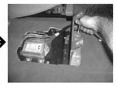
**STEP 22:** Remove the OEM console bracket, that is mounted to the floor.
