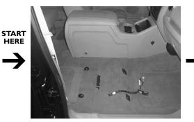
\*Caution\* You may be working on a Expedition that has side air bags, located in the front seats. We do ask for the removal of these front seats. Disconnect the negative side of the battery and leave for 15min. This will allow for discharge of the air bags. Once the air bag wires have been disconnect, do not turn the ignition on. If you do, the computer will present an air bag fault. You may try to accomplish this install, by not removing this seat.
