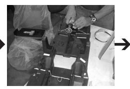
**STEP 17:** Cut the black inner console, following the scribe lines. A jig saw, air saw or cutting wheel can be used.
