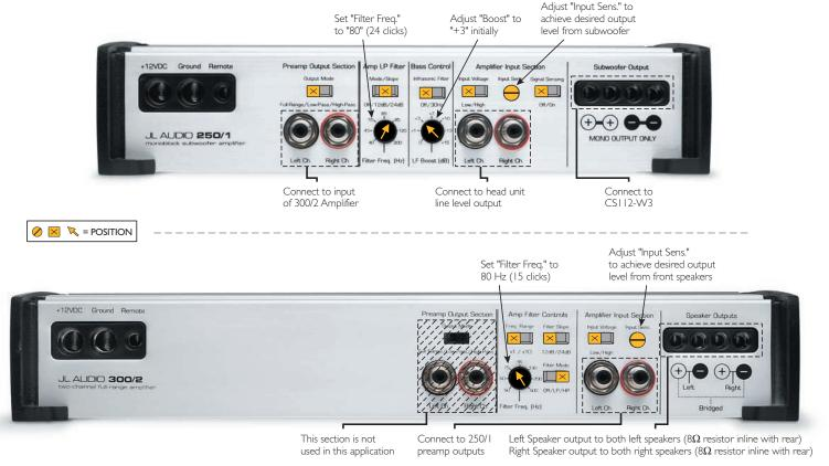
**Note:** These settings are intended as a "baseline" for tuning this system. Depending on the vehicle and the customer's tastes, some variation in the crossover and bass control settings may be necessary for optimum performance.
